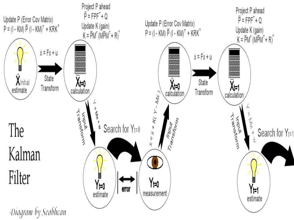
The Kalman filter is an algorithm that uses <u>a series of</u> <u>measurements observed over time</u>, containing noise (random variations) and other inaccuracies, and produces estimates of unknown variables that tend to be more precise than those based on a single measurement alone
