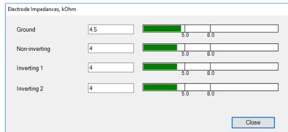
**Figure 14.** Check Impedance Dialog Box (G2 System)
