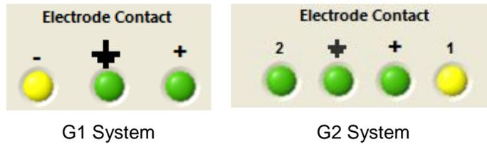
Figure 9. Poor Electrode Contact
