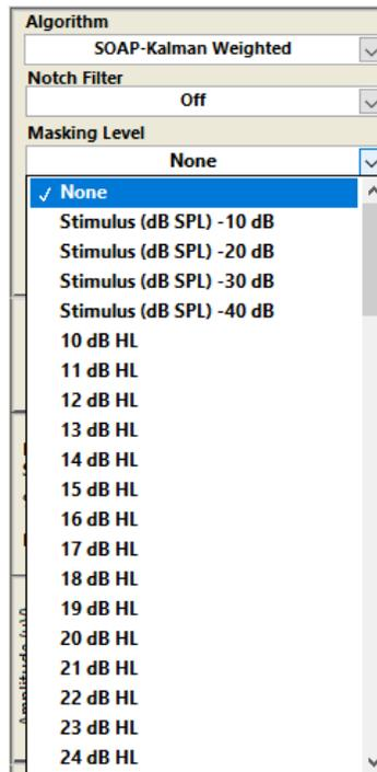
**Figure 49.** Masking Level drop-down on Test Screen
