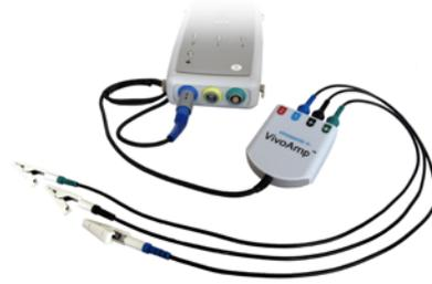
**Figure 121.** 3-leads with alligator electrode clips
