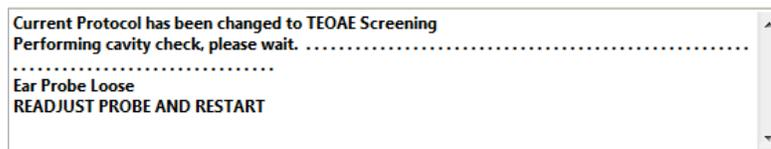
**Figure 97.** Probe-check message - Readjust
